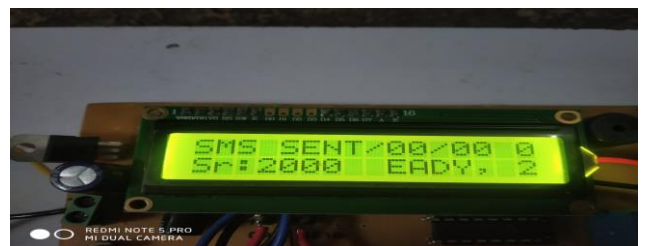
Fig 3.2 LCD displaying Sr. no. and message sent on display.
