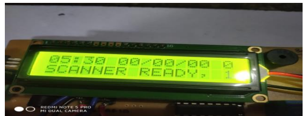
Fig 3.1 LCD “displaying scanner ready” indication
