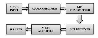
Fig 6: Block Diagram of Audio Communication
