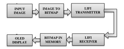
Fig 5: Block Diagram of Image Communication
