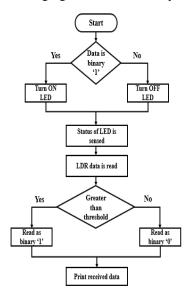
Fig.2. Flowchart of Li-Fi communication
