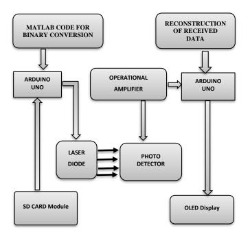
Fig 3: Block diagram of Li-Fi Communication system
