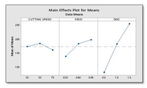
Fig. 4. Graph Effect of turning parameters on the multiperformance characteristics.
