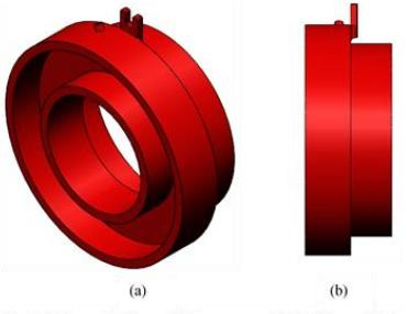
Fig.1. Shows the Isometric view and Side view of the Stator.
