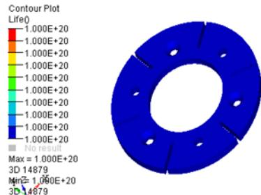
Fig.15. Fatigue Analysis of Armature
