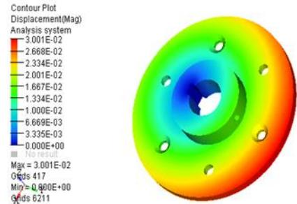
Fig.13. Total Deformation in Flange
