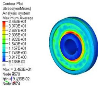
Fig.8. Total Stress in Rotor
