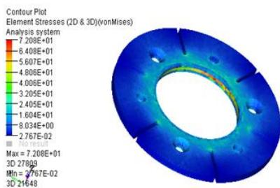
Fig.10. Total Stress in Armature
