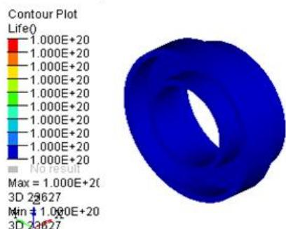
Fig.14. Fatigue Analysis of Stator
