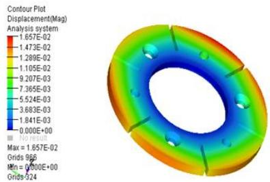
Fig.11. Total Deformation in Armature
