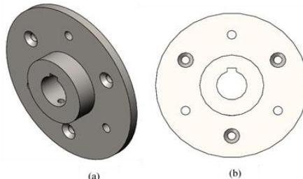
Fig.5. Shows the Isometric view and Side view of the Flange.
