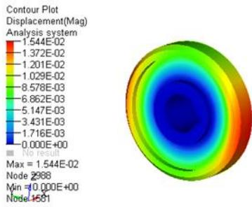
Fig.9. Total Deformation in Rotor
