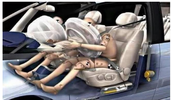
Fig.2. The working principle of air bag
