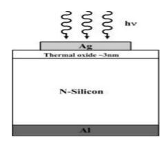
Fig.6. Structure of metal oxide semiconductor using UV sensor
