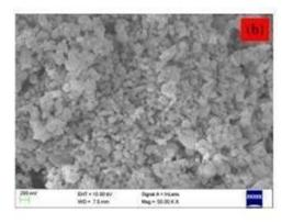
Fig.13. (b) Field emission scanning electron microscopic analyzes (b) Co doped ZnO nanoparticles [22]
