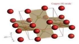
Fig.17. Crystalline structure of CuO [27]
