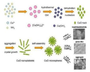
Fig.18. Formation of different CuO nanostructures [26]
