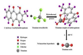
Fig.14. Mechanism of TiO2 nanoparticles [24]
