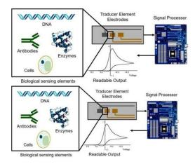
Fig.5. Biosensor coupled with electrodes [11]
