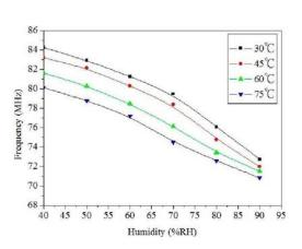
Fig.4. (a) Humidity sensor b) capacitance of humidity sensor at different temperature c) output frequency [9][10]
