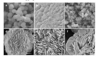
Fig.19. SEM image of different CuO nanostructures in different concentration [26]
