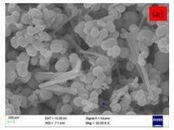
Fig.13. (a) Field emission scanning electron microscopic analyzes (a) Pure ZnO [22]
