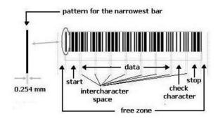
Fig.8. Barcode Structure
