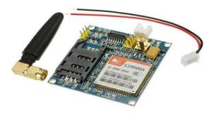
Fig.3. GSM Module
