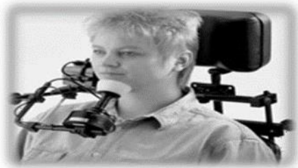
Fig.2.4. Power wheel chair chin-operated force sensing joystick
