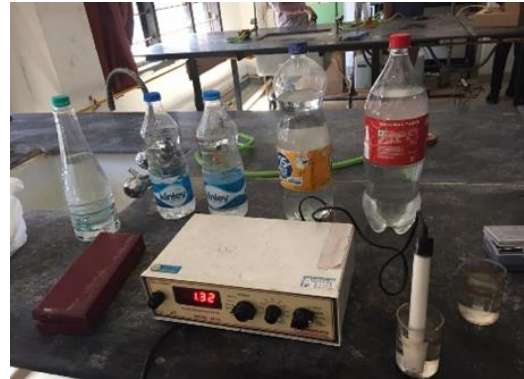
Fig.3. Determination of conductivity of water
