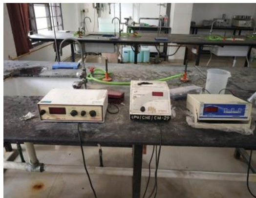
Fig.4. Determination of dissolved oxygen (DO) of water
