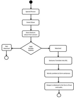
Fig 3.5. Activity Flow Diagram
