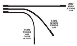
Fig. 5.5. Flex Sensor and its Bending
