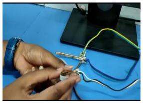
Fig 5.12. Testing of reliability of flex sensor
