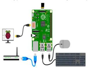
Fig .5.7. Block Diagram of Conations for Peripheral Devices
