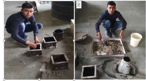
Fig.1. Preparing of cubes in laboratory and mixing of concrete
