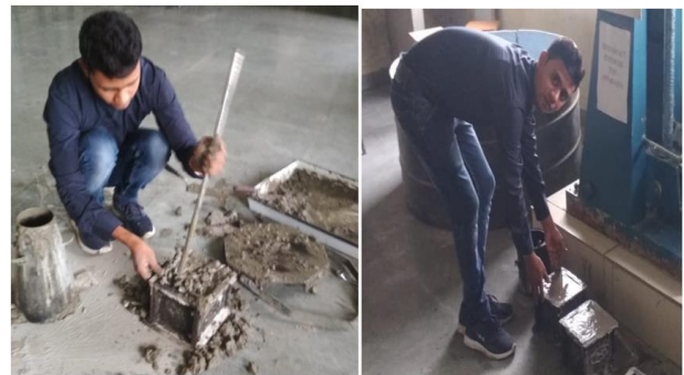
Fig.2. Moulded of cubes in laboratory
