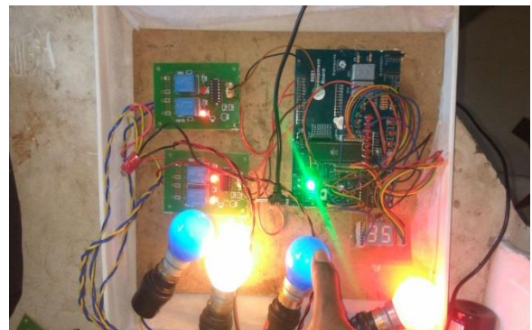
Case4: All the four bulbs are in ON condition when count is greater than 30 and less than 50.
